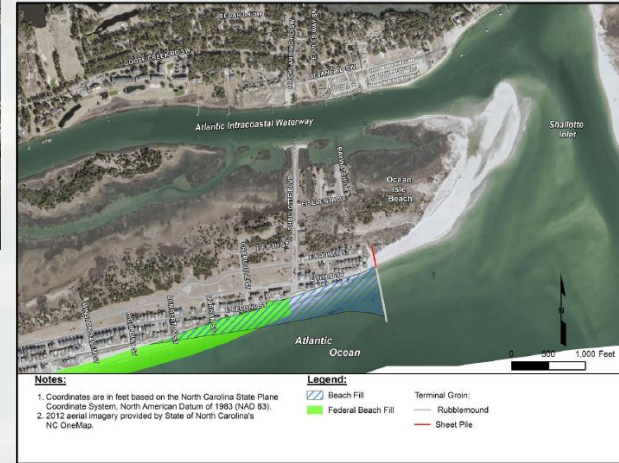
Armoring or modifications to beach fill
